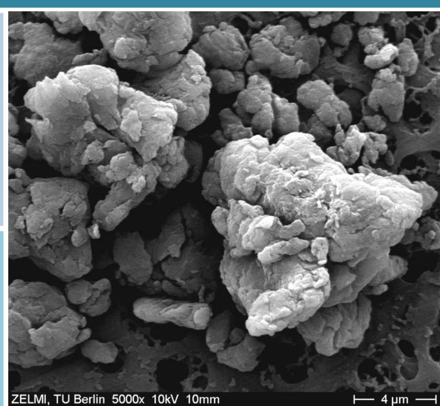
Electron micrograph of the used polystyrene microplastics (© TU Berlin)
